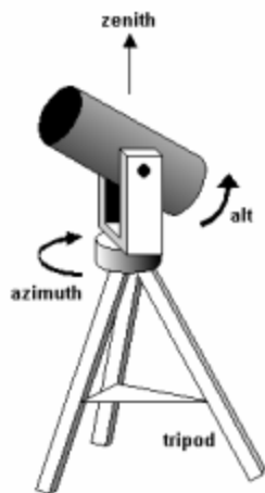
Figure 3—Alt-Az Fork Mount Fork mounts are easily motorized for tracking and commercial ones for larger scopes typically are. Since it's necessary to track simultaneously in both axes, there are two sets of motors and worm gears. One will be mounted in the base of the mount to rotate in the azimuth axis and the other is mounted in one or the other fork arm to rotate in the altitude axis.
